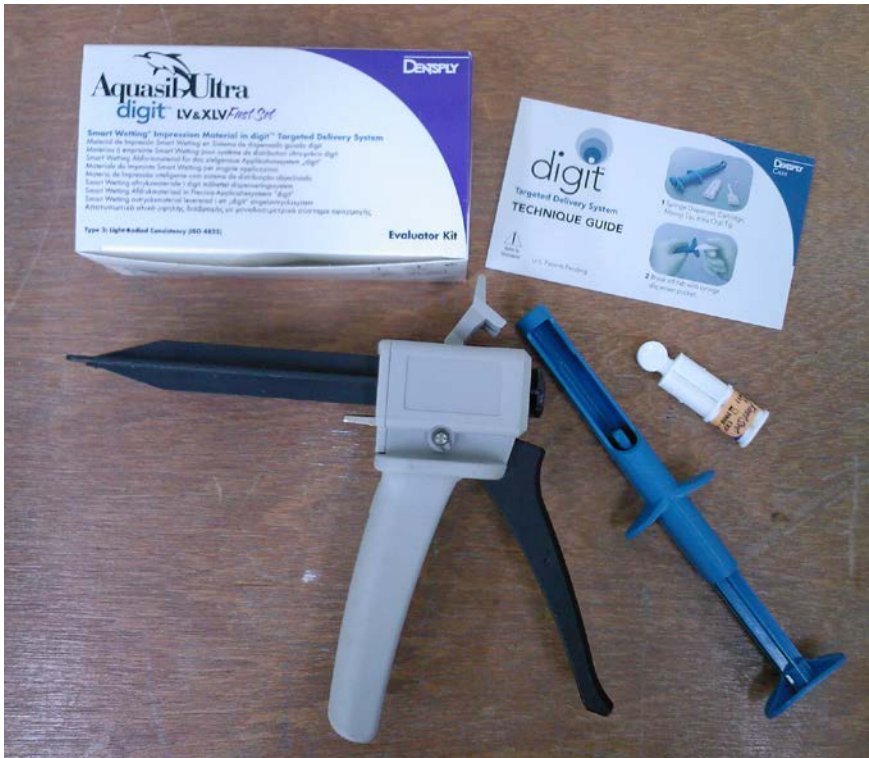
Aquasil silicone gun for the application of a silicone mould to recreate texture. (Image credit: Kate Seymour, SRAL)
