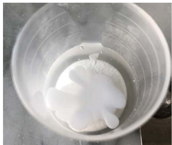
Liquid ingredients are measured and mixed thoroughly before adding the dry components. Liquid ingredients are methylcellulose (Methocel A4M) and Evacon R (Preservation Equipment)
