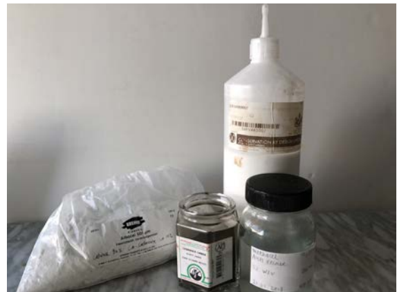
Ingredients needed for a lightweight filling with methylcellulose, Evacon-R, Arboce 500, Aluminium hydroxide and pigment.
