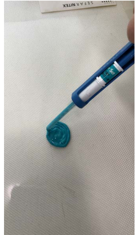
The mould is put in the gun and the two-part components are mixed and applied to a textured surface. (Image credit: Kate Seymour, SRAL)
