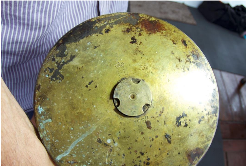
Figure 30: Base markings 15cm cartridge case from the Java site. Note the Dutch crown and manufacture date 1922.
