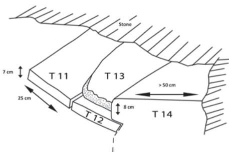
Fig. 25: Schematic drawing of H3: keel, rabbit and shell planks
