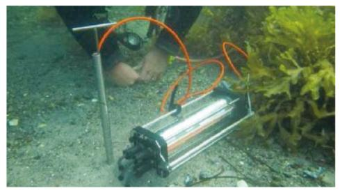
Fig. 23: The spear-like sediment profiler tested at Tudse Hage.
