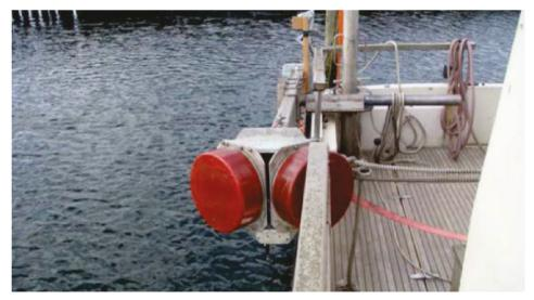
Fig. 2: Example of a MBES system
