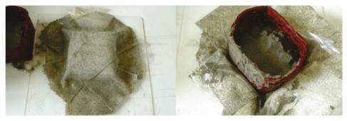
Fig. 37: The 3M™ Scotchcast ™ Plus Casting Tape tested in laboratory. Photo MBACT - ISCR
