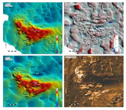
Fig. 18: Comparison between multi-beam surveys from December 2013 and September 2014. At the top left is the multibeam of 2014; lower left, the multi-beam of 2013. The top right shows the difference in sedimentation; red indicates incline, blue a decline. The lower right is a side-scan sonar picture from September 2014.
