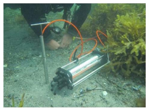
Fig. 10: The diver-operated datalogger with spear sediment profiler.
