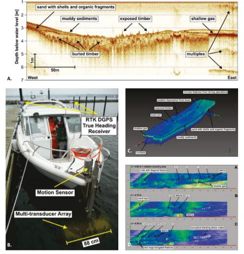
Fig. 6A: Parametric sub-bottom profiler seismic section from the central region of the study area near Schleswig (Northern Germany) showing several reflectors caused by sediment boundaries, a locally confined (South East) high amplitude reflector caused by a shallow gas layer, numerous small diffraction hyperbolas and some short linear reflectors caused by exposed and buried objects. Time to depth conversion was performed with a constant velocity of 1500 m s-1. Vertical exaggeration = 16:1.
