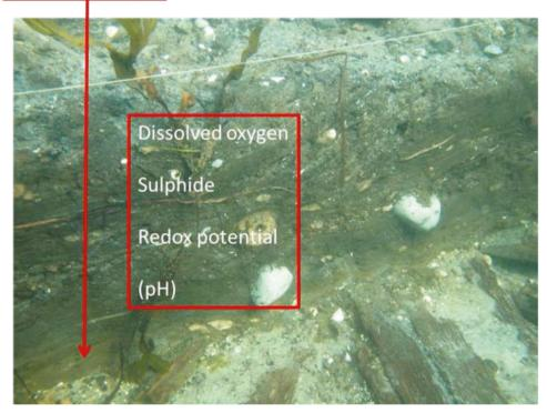
Fig. 24: In situ profiling to characterise whether a site is oxic or anoxic.
