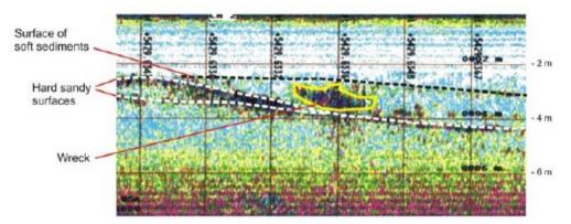
Fig. 5: The Haithabu wreck found by using a sub-bottom profiling system.
