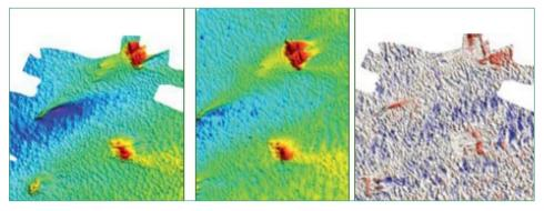
Fig. 21: Multi-beam images of the BZN 10 wreck in 2003 and 2004, and a map which shows the changes in sediment.
