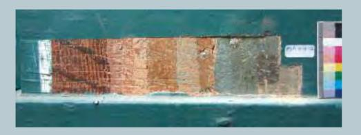
84 Stratigraphic study of the exterior of one of the ressaults of the partitions of the women's galleries. The paint layers have been exposed one by one with a surgical scalpel; this provides an image of all the different paint layers that are present, from the most recent one (on the left) to the earliest grey finishing layer (on the right).
